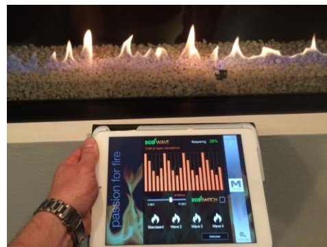
11 – To get to the screen of the Eco Wave Settings, you press on your device with the Eco Wave Text of picture 10
