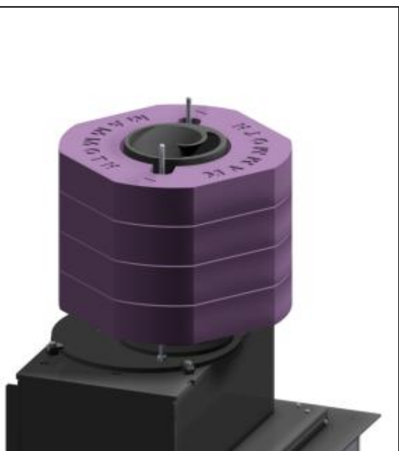
5. Placing other brick segments
