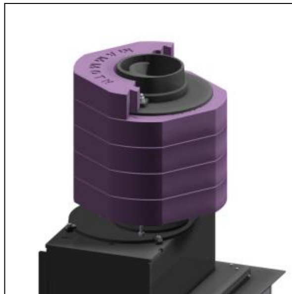
7. Then last brick segments are installed to complete the set.
